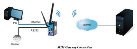
The gateway provides a variety of VPN security connections and supports server and client mode in VPN connection.
